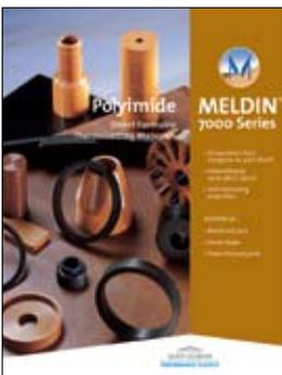
Premium polyimide direct formable materials suitable for high volume production, for use in 600°F (316°C) or lower applications. Available in custom finished parts only, except as noted.
